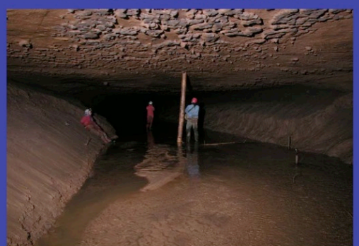
Major cave stream (Logsdon River) in Mammoth Cave, showing the base of a 145-m-deep monitoring well. The stream at this point drains the groundwater flow from an area of about 27 km 2
